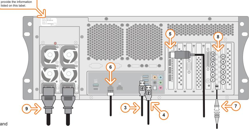
8 Connect the HD-BNC end of the pigtail cables to the HD-BNC connectors and attach the SDI cables to the BNC end of the pigtails according to their required destination (see the *XPression User Guide* or Help file for information about configuring the key and fill for the HD-BNC connectors).
